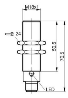
Inductive Sensors BES 516-212-E5-E-S 27 M18x1 x 70.5 normally-closed Sn=5mm shielded
